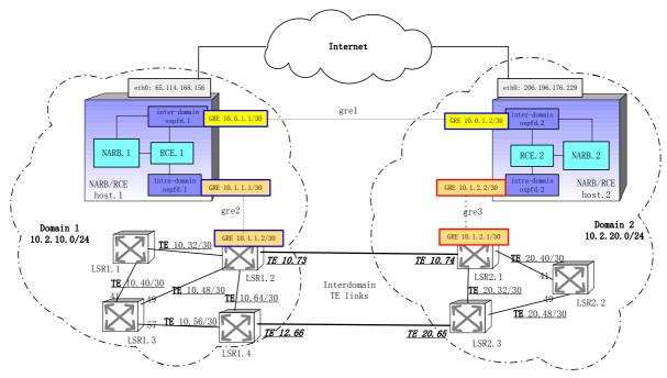
Figure 4: An example two-domain network configuration.
