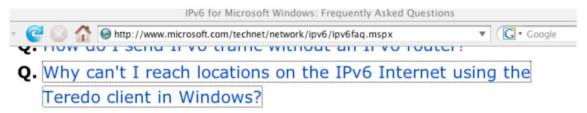
A. To reach the IPv6 Internet from behind a network address translator (NAT) using the Teredo client included with Windows, there must be an operational Teredo relay attached to the IPv4 and IPv6 Internets. At this time, Microsoft is not providing any operational Teredo relays for reachability to locations on the IPv6 Internet for Windows-based Teredo clients.
